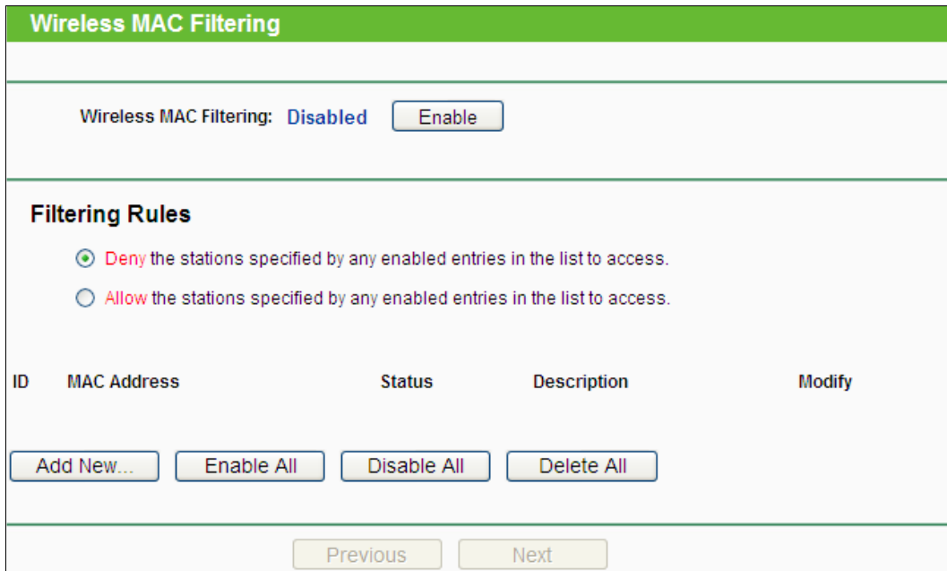
Figure 4-20 Wireless MAC address Filtering
