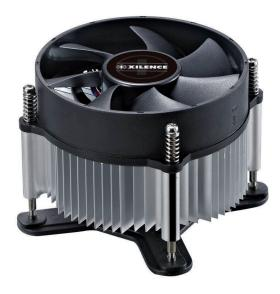
The Xilence I-110 combines all features of a current CPU cooler for home and office. Thanks to the quiet-running 92mm fan the precisely manufactured heat sink gets reliable and quiet cool air all time. The fin design not only ensures efficient cooling of the CPU, but also cools all surrounding components. The fan speed of 2200rpm guarantees an ideal compromise between high air and quiet operation. This is why the Xilence I-110 is a very interesting Intel cooler in the beginner area.
