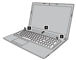
**6** Lift up the keyboard **4** and detach the connector in the direction shown by the arrows **5 6** .
