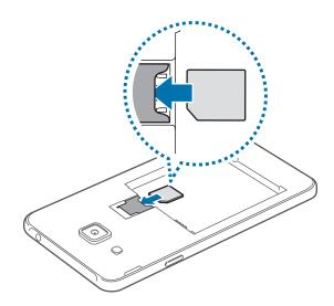
▶ **Dual SIM models**: Insert the SIM or USIM card with the gold-coloured contacts facing downwards.
